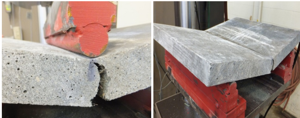
Figure 4.20 Testing of reference panels made with 2% steel microfiber
