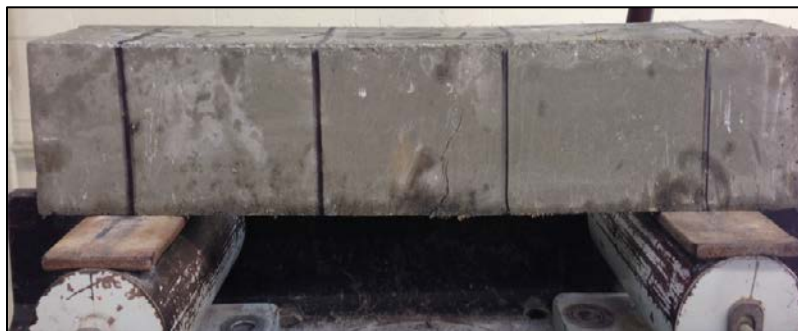
Figure 3.44 Failure configuration after test
