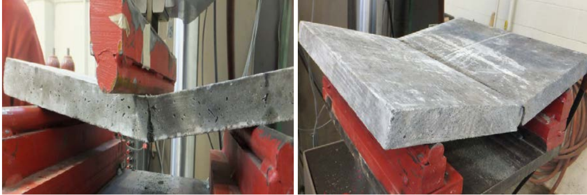
Figure 4.18 Failure mode of panels with GFRP type II grids
