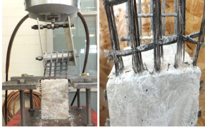
Figure 4.8 Failure mode of bricks with two layers of GFRP grids
