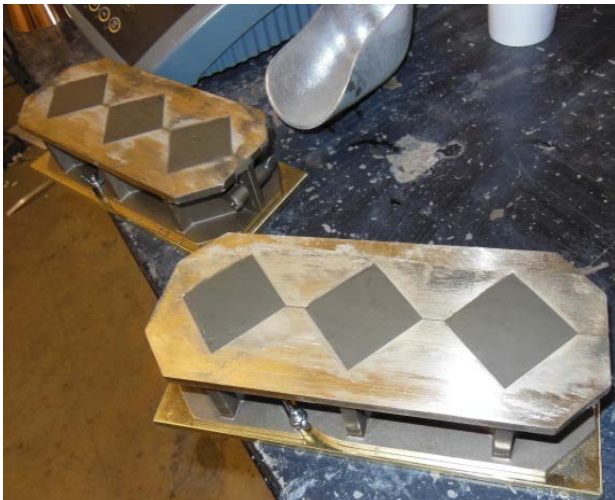
Figure 3.9 Compressive strength test sampling
