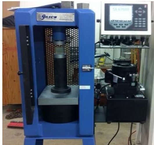
Figure 3.10 Compressive strength test set-up
