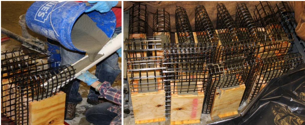
Figure 4.5 Bricks with FRP grids embedded for pull-out test
