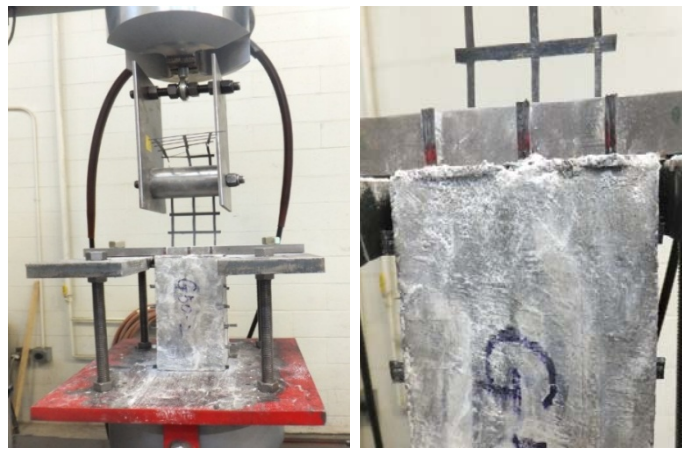
Figure 4.9 Failure mode of bricks with one layer of CFRP grids
