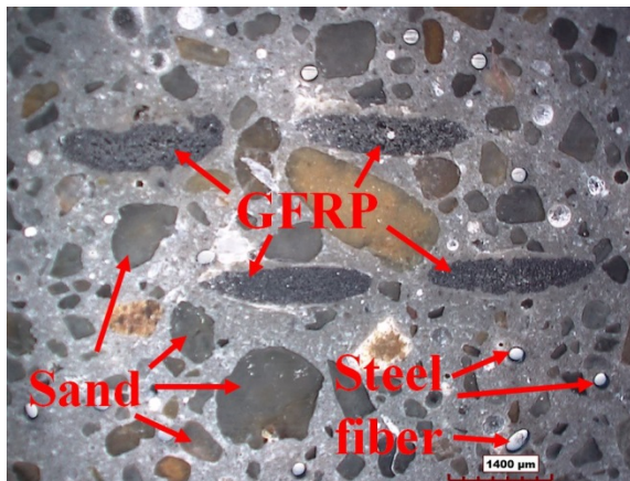
(a) 2 layers of GFRP
